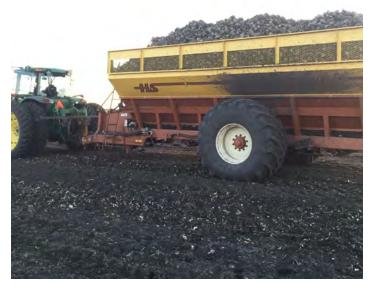
Many farms use a beet cart to help keep the harvester going and reduce truck traffic in the field. It also helps when conditions are muddy and the trucks cannot travel in the field
