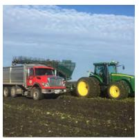
hopper. The hopper cannot store very many sugarbeets so usually the truck comes right alongside the harvester, and takes beets immediately. Some operations use a beet cart, which is similar to a grain cart.
